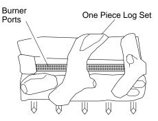
Figure 19 - Installing Heat Majic™ One-Piece Log Set (Top View)
